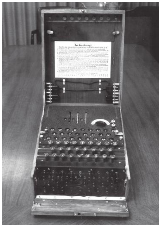
FIGURE 2.3 (a) Enigma rotor assembly. (b) A World War II enigma cipher coding machine. (Both images courtesy of Shutterstock.com.)
